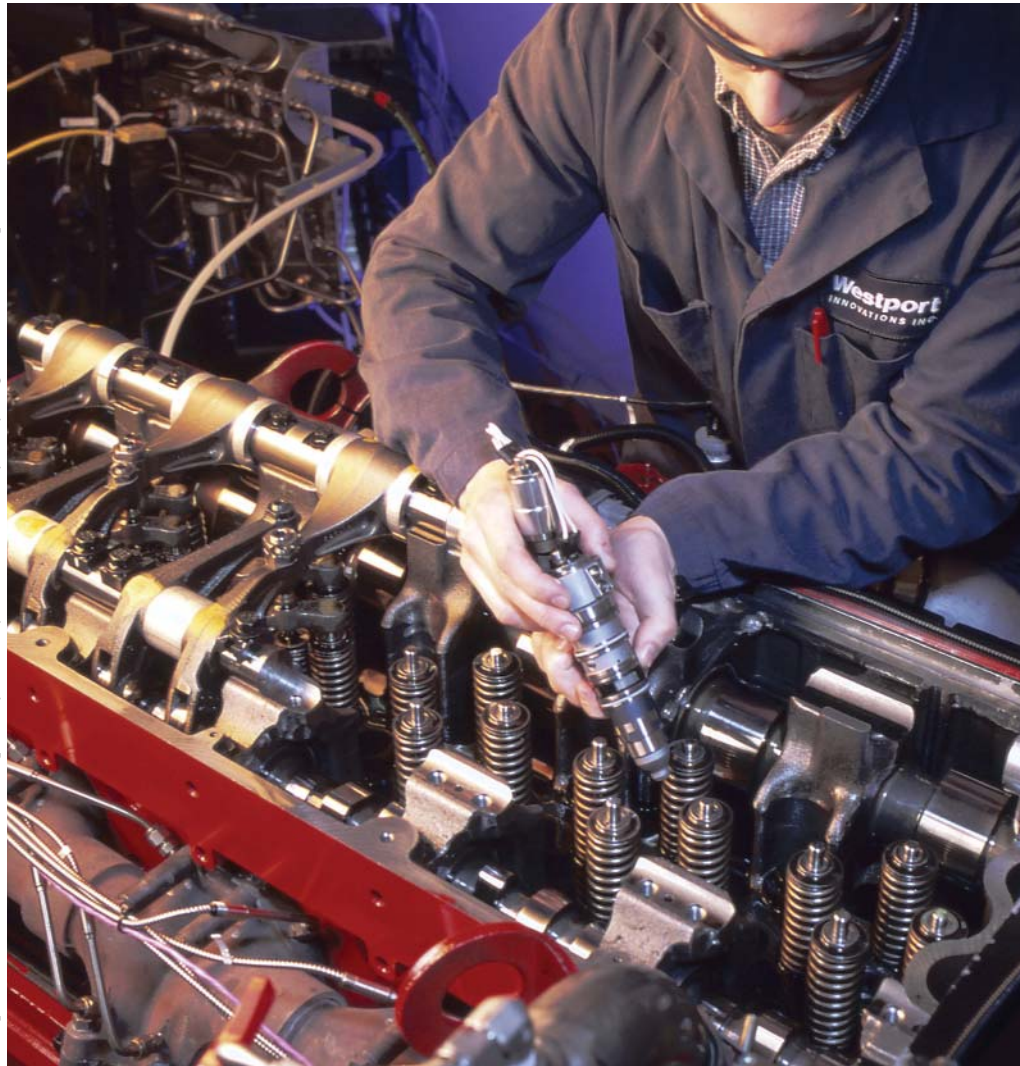
Westport technician installs a Westport-Cycle™ injector into a heavy-duty engine. Photo: Westport Innovations Inc.
